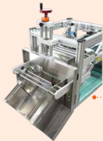
合格品收料槽 (收料槽寬度 / 高度可調) Collection tray for acceptable products (Width / Height adjustable)
