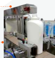
瓶口壓制機構 Bottle hold down device 進瓶導正系統 Bottle feeding servo-alignment system
