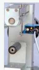
軟管貼標模具 & 貼標定位電眼 (選配項目) Tube mold & Label positioning sensor (optional items)
