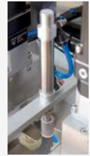
壓蓋穩定裝置 Capping stabilization device
