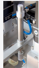
壓蓋穩定裝置 Capping stabilization device
