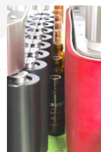
連動式扶瓶機構 Interlocking bottle clamp
