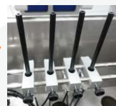
氣洗噴頭 Air-rinsing nozzles
