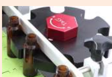
星盤式分瓶裝置 Indexing bottle separation device
