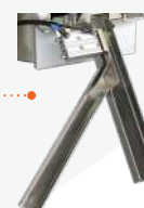
漏標自動剔除裝置 Automatic rejection device for missing-label product
