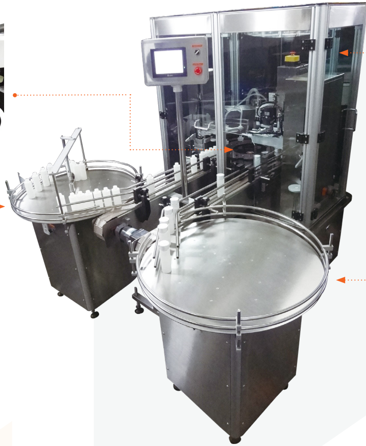
機台安全外罩 Machine safety cover
